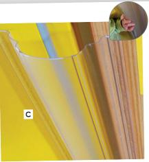
HINGE PROTECTOR Easy to install with adhesive strips (supplied). Designed to withstand 250,000 openings and closings of a door. Consists of: 1 wide strip (for placing on the hinge pin side of the door) and 1 narrow strip (for placing on the hinge side of the door). Made from PLASTIC.
